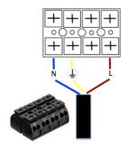
(Incoming supply wiring schematic – Input Cable max 1.5mm², 3 core must be tethered to P-Clip)
