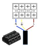
(Incoming supply wiring schematic – Input Cable max 2.5mm<sup>2</sup>, 3 core must be tethered to P-Clip)
