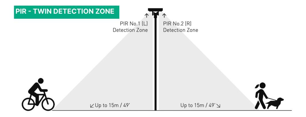
The first solar lantern built for Britain, the DEFENDER-55 is the most advanced medium duty solar light available. Featuring adjustable angle LED's, twin PIR motion detection system and advanced nano-particle battery technology with fully programmable solar controller.
